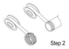
3. Screw pipe into bushing.
