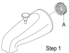
2. Wrap Teflon tape on both bushing and pipe. (Considering the different Teflon tapes are with different thickness, please wrap Teflon tape at least 6 cycles. It would be better to wrap more than 6 cycles.)
